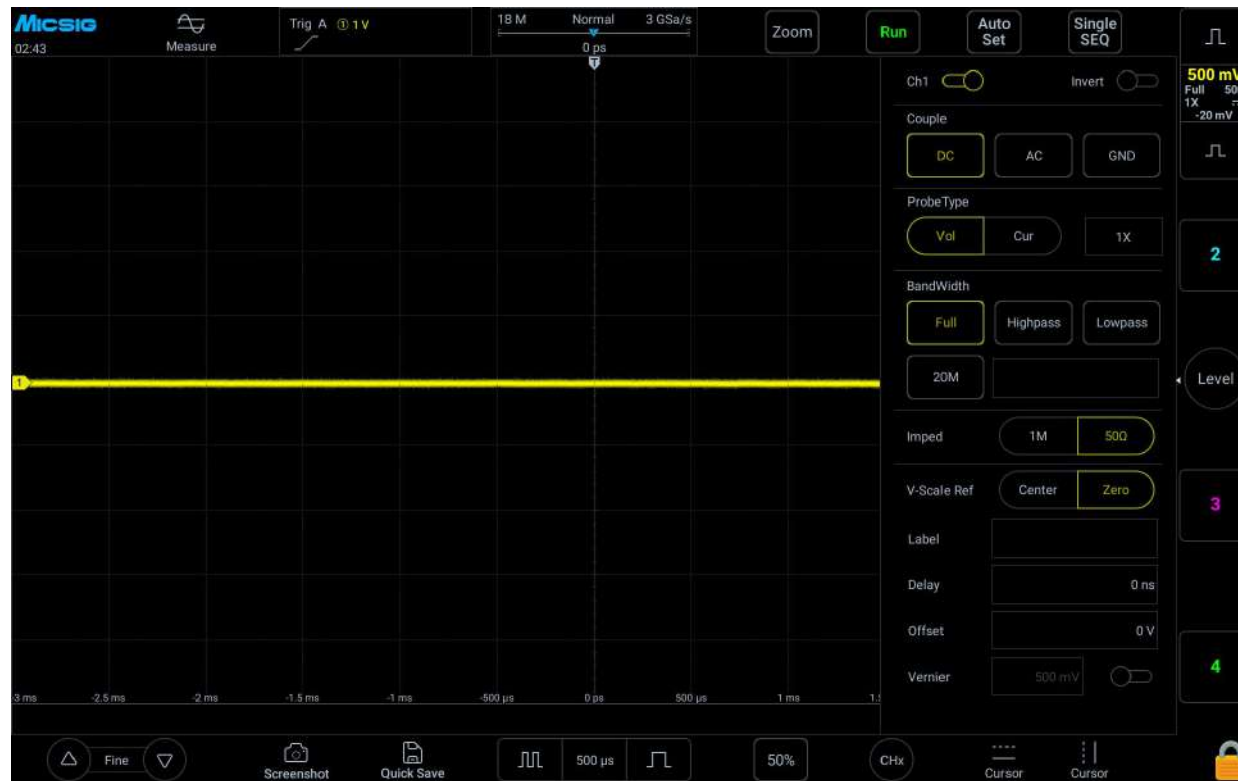
Figure 4-17 Channel input impedance
