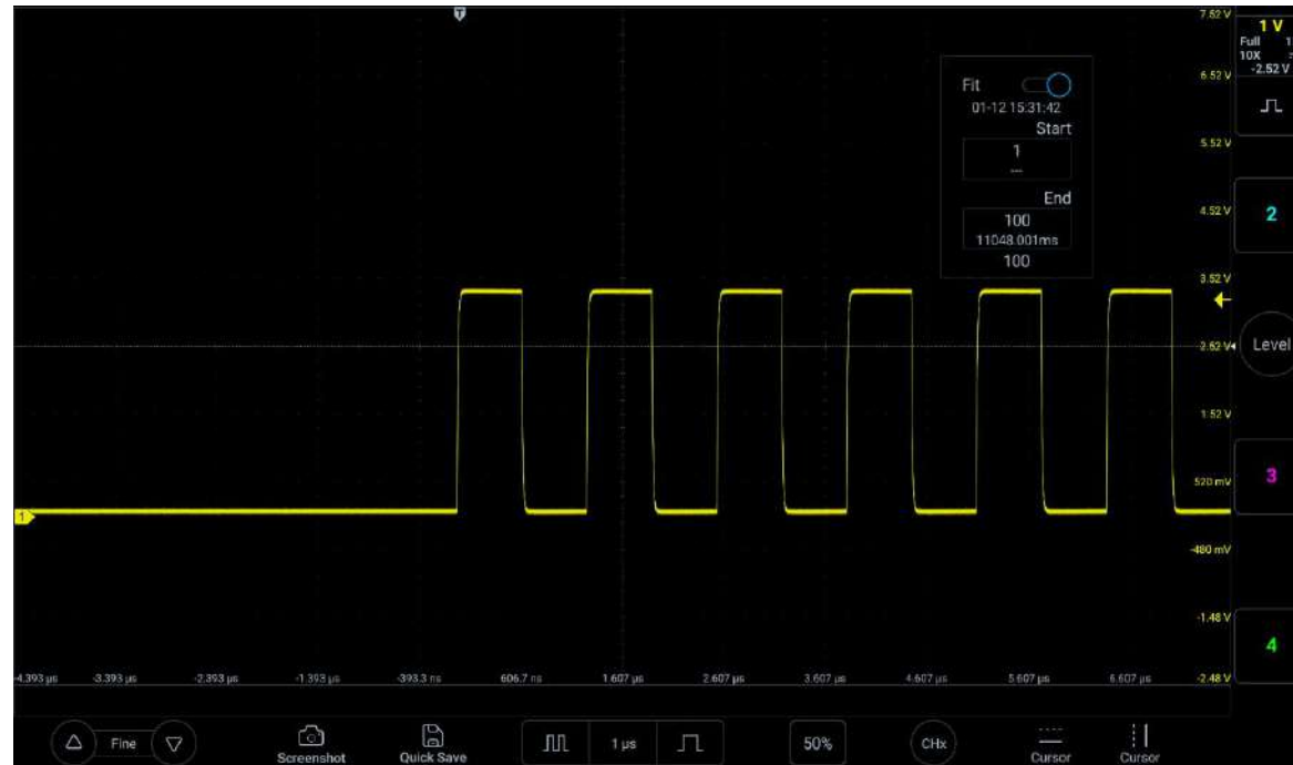
Figure 10-13 Segmented storage fitting view
