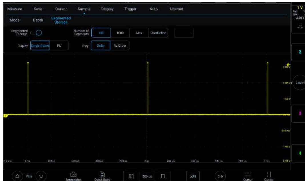
Figure 10-11 Segmented storage waveform acquisition
