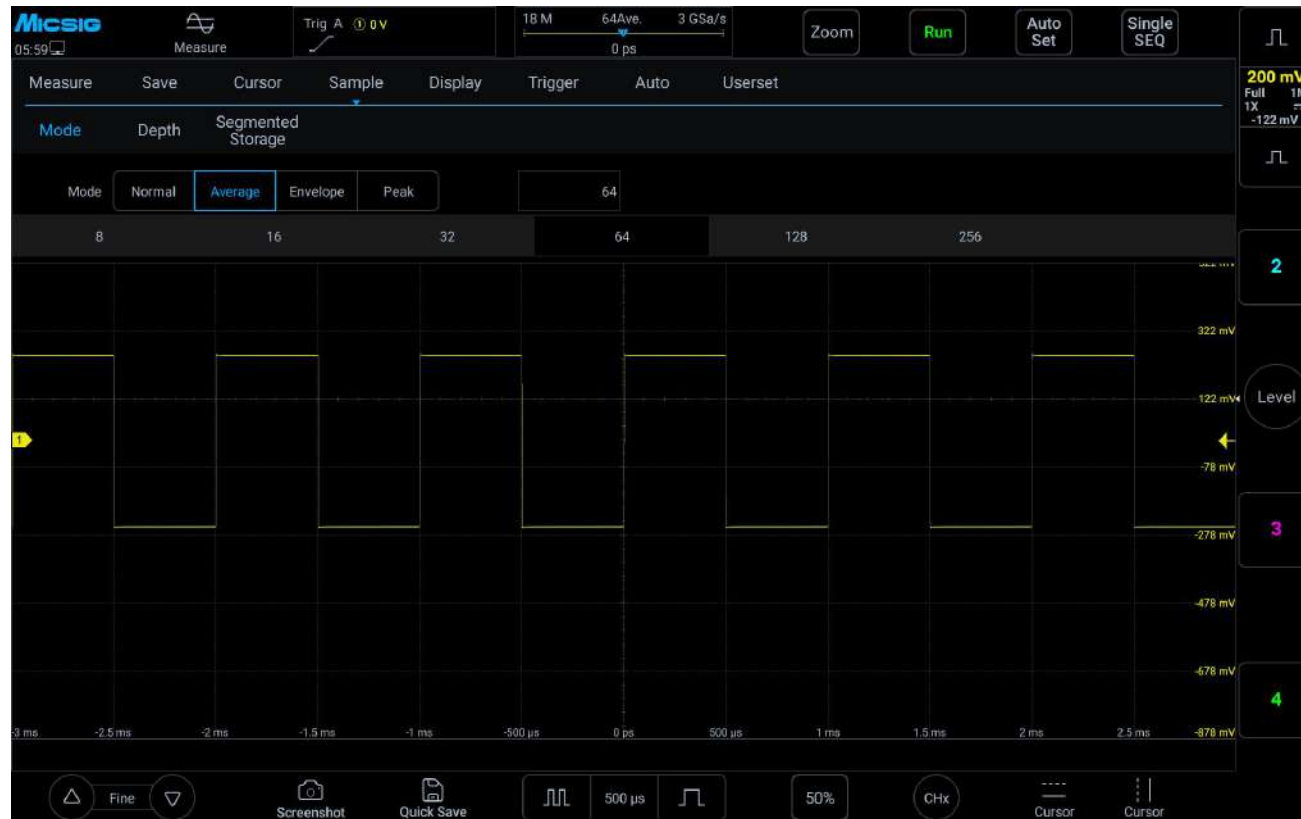
Figure 10-7 Waveform after choosing the average sampling mode, with average number 16
