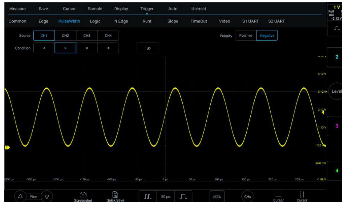
Figure 5-15 Negative Polarity Pulse Level Flip
