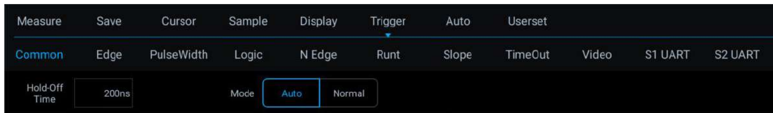
Figure 5-5 Oscilloscope Trigger Mode Setting
