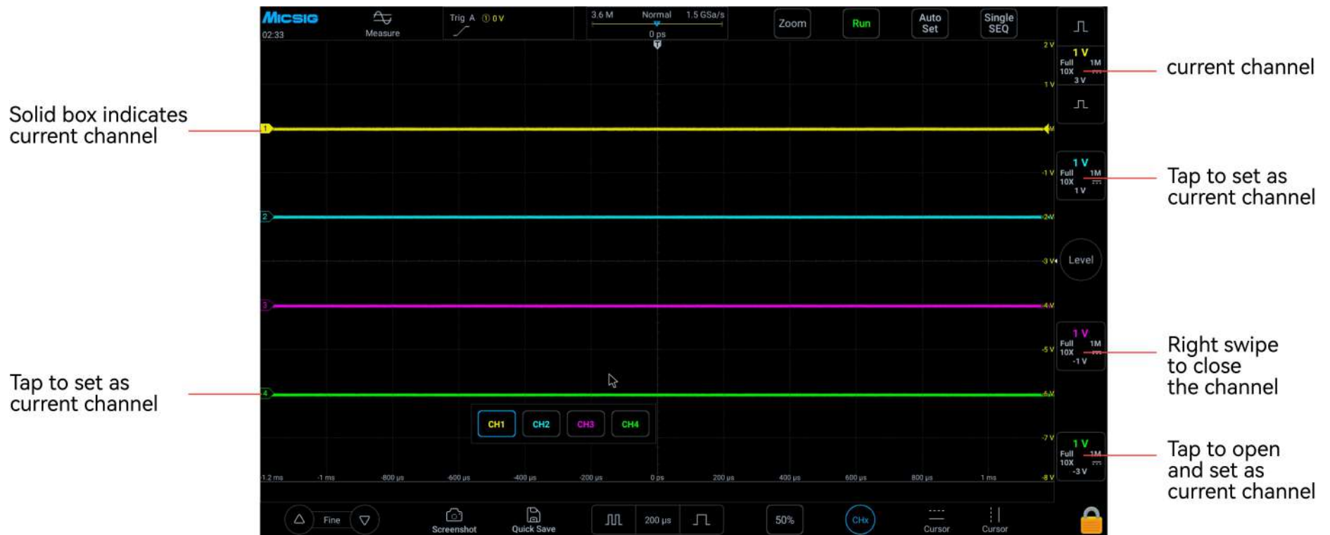
Figure 4-4 Channel Open, Close and Switching
