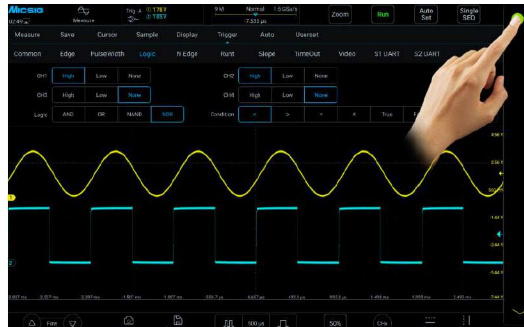
Figure 5-22 Trigger Level Adjustment
