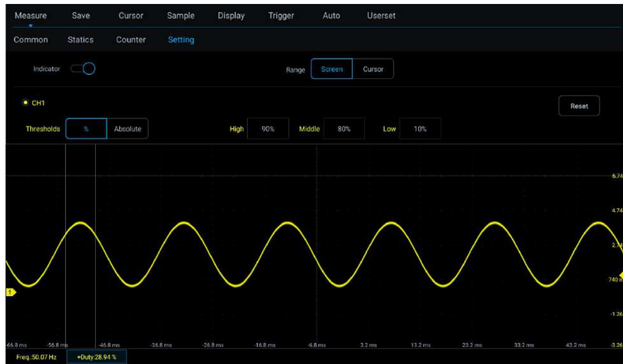
6-13 Pulse width when the median threshold value is set to 80%
